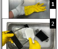
Step 5: Wash, rinse, and sanitize the unit and parts using a brush handle. Note: Take safety precautions by wearing cut gloves underneath rubber gloves. (See Diagram 1)
