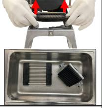
Step 4: When finished processing food, remove the blade carefully using cut resistant gloves and place the T handle/pusher block unit and blade assembly in a hotel pan for safe transportation.
